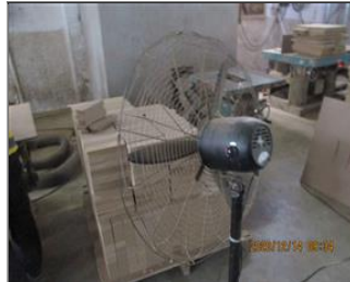
Photo of non-conformity The gap between the metal frames of all fans used in workshops is about 2cm.JPG
