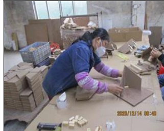
Photo of non-conformity 1 gluing worker only wear dust mask instead of effective active carbon mask.JPG
