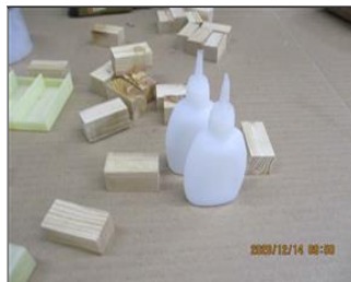
Photo of non-conformity no safety label for glue used in assembly workshop.JPG
