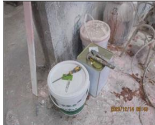
Photo of non-conformity no safety label and secondary containment was available for chemicals used at spraying workshop such.JPG
